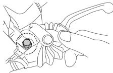
The pivoting points of the front and rear brake levers must be lubricated at the intervals specified in the periodic maintenance and lubrication chart. Recommended lubricant: Silicone grease
