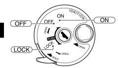
The main switch/steering lock controls the ignition and lighting systems, and is used to lock the steering. The various positions are described below.
