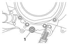
1. Engine oil drain bolt A
