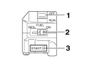
1. Engine stop switch "ENGINE STOP"
