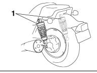
1. Shock absorber assembly  $(\times 2)$
