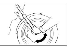
Hold the lower ends of the front fork legs and try to move them forward and backward. If any free play can be felt, have a Yamaha dealer check or repair the steering.
