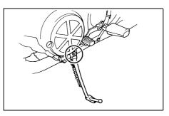
Recommended lubricant: Lithium-soap-based grease (all-purpose grease)
