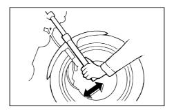
Hold the lower ends of the front fork legs and try to move them forward and backward. If any free play can be felt, have a Yamaha dealer check or repair the steering. **Checking the wheel bearings**
