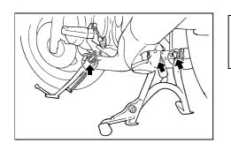
Recommended lubricant: Lithium-soap-based grease (all-purpose grease)
