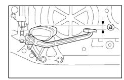
a. Distance between brake pedal and footrest
