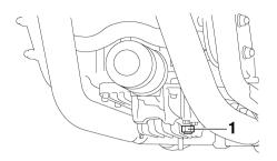
1. Engine oil drain bolt
