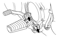
The operation of the brake and shift pedals should be checked before each ride, and the pedal pivots should be lubricated if necessary.
