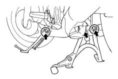
The operation of the centerstand and sidestand should be checked before each ride, and the pivots and metal-to-metal contact surfaces should be lubricated if necessary.
