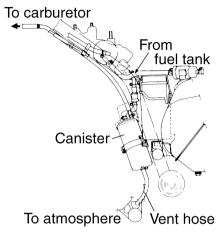
This model is equipped with a canister to prevent the discharging of fuel vapor into the atmosphere.
