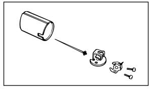
8. Remove the float chamber by removing the screws.
