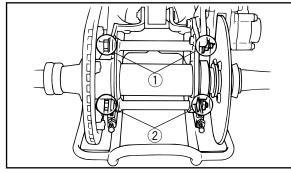
1. Upper wheel hub bolt (x2) 2. Lower wheel hub bolt (x2)
