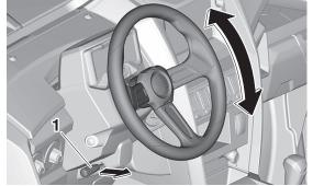
1. Steering wheel position adjusting lever
