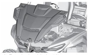
2. Turn the hood locks 1/4 turn counterclockwise, and then push the tab on each hood lock down so that it is pointing rearward. Make sure that the hood is securely installed.
