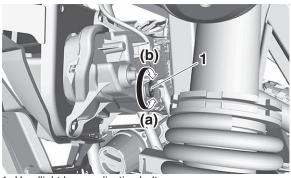
1. Headlight beam adjusting bolt
