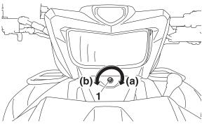
1. Handlebar-mounted light beam adjusting screw
