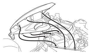
2. Install the screws, quick fasteners, bolts, and hoses.
