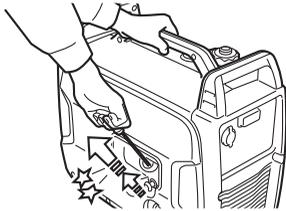
**5.** Grasp the recoil starter handle and pull slowly until resistance is felt. Give the starter handle and rope a short, brisk pull to start the engine.
